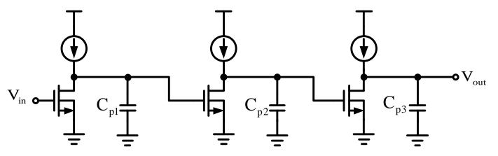
• The parasitic load capacitance at the output of the i<sup>th</sup> stage is approximately given by  $C_{pi} \cong C_{0-i} + C_{gs-i+1}$
