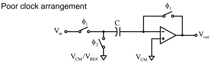
•  $V_{in}$  needs to charge C during  $\phi_1$  is high
