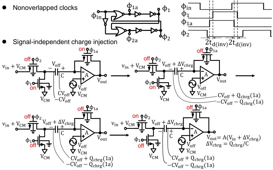
Constant charge-injection error can be treated as a DC signal and thus can be ignored in most signal processing applications.
